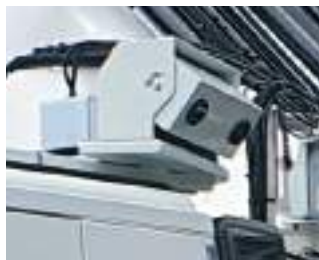
Stereo camera installed on both sides of lorry cab.
