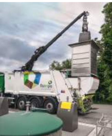
Container emptying by means of roof crane with Speed-Gripper.
