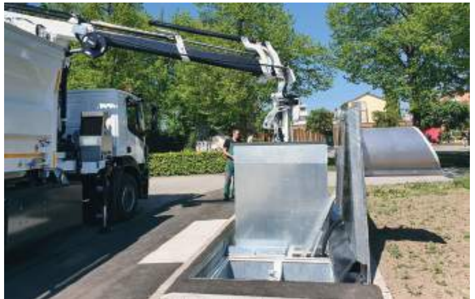
The steel container of capacity 6 m 3 is emptied by the Speed-Waste-Lifter.
