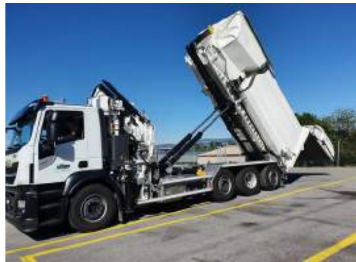
Emptying the compactor container
