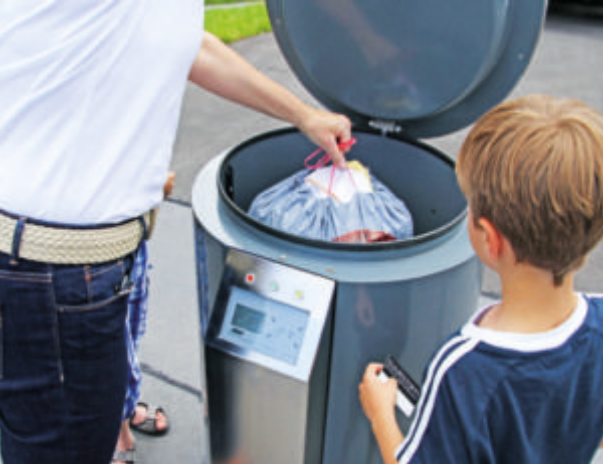
Residual waste disposal, Caslano type throw-in column with weighing
