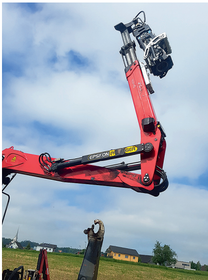
Position the telescopic arm vertically and drive into the console.
