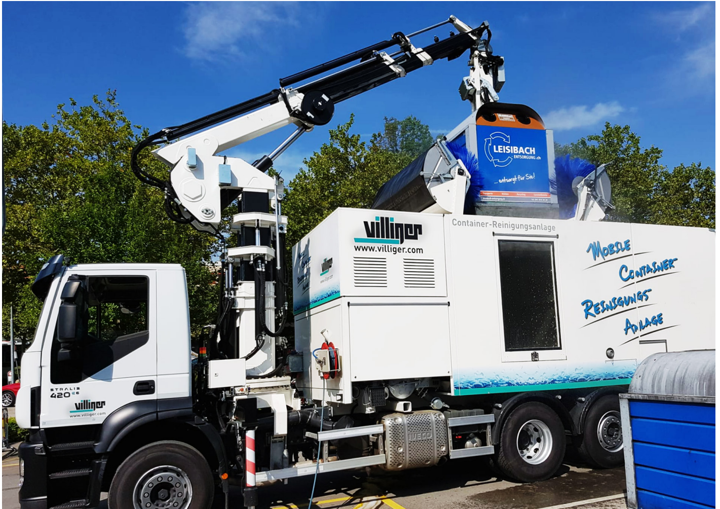
Mobile cleaning system for the exterior and interior cleaning of an above-ground container.
