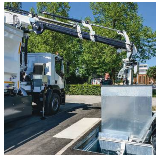
Emptying of steel container with a capacity of 6 m 3 by a Speed-Waste-Lifter.
