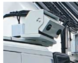
Stereo camera installed on both sides of the truck cab.
