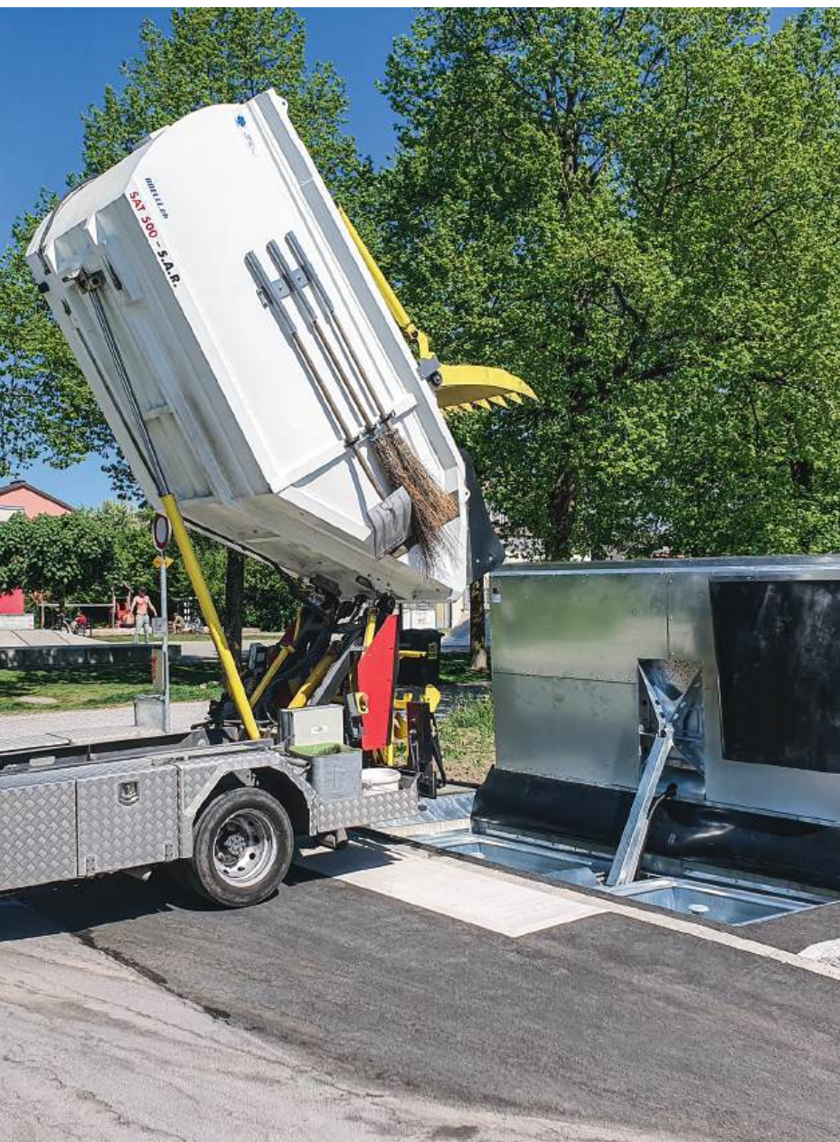
Unloading of a tipper into a Swing-o-Mat system SW 400.
