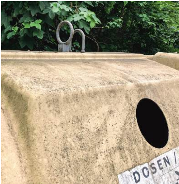
Container with 2 hooks pickup system before retrofit ...
