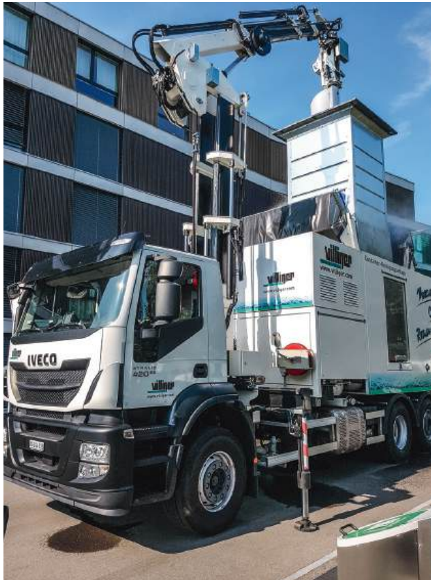
Automatic washing of an underground container in the mobile cleaning device.
